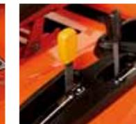
Hydraulic mower lift lever
