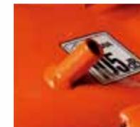
Deck cleaning pipe for connecting water hose
